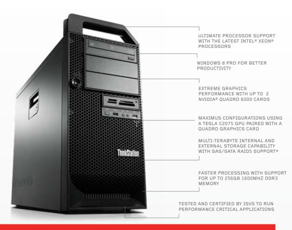
Unveiling the Lenovo® ThinkStation® D30 workstation – extreme performance machines designed for highend professional computing. Experience the latest fast running Intel® Xeon® eight core processors and high-performance dual NVIDIA® Quadro graphics. The ThinkStation® D30 is designed for professionals who demand the ultimate in performance and reliability.
